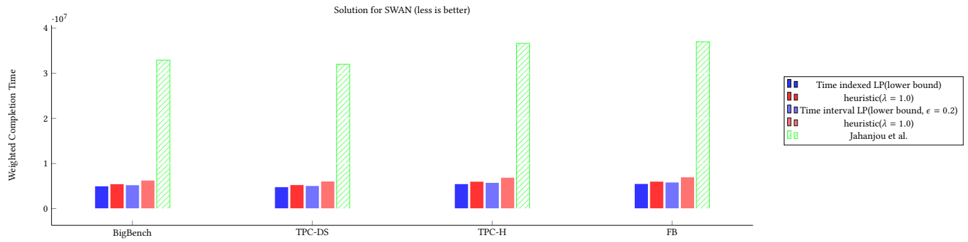
Figure 9: Single path model on SWAN, showing the performance bound of time indexed and time interval LP value, the performance of heuristic ( \lambda = 1 ), best \lambda among samples, and the expected value when \lambda is chosen from the distribution mentioned in Section 4.1. Here we compare against algorithm by Jahanjou et al.[15].
